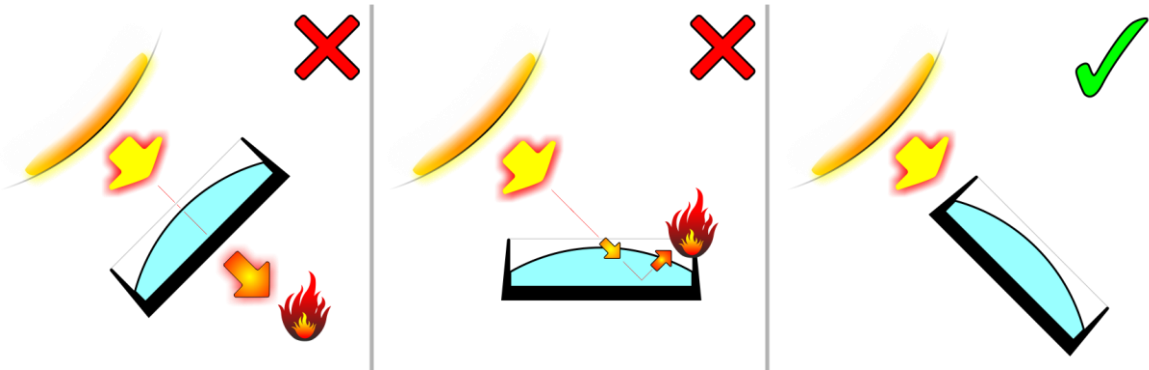
Figure 1. Avoiding damage from light sources
