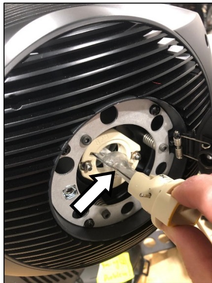
Figure 8. Metal rod on lamp must face upwards
