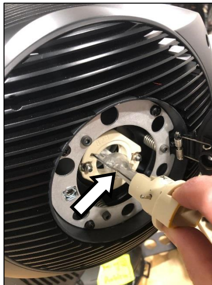
Figure 8. Metal rod on lamp must face upwards
